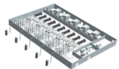
100 MW Solution (10 x 10 MW Electrolyser Stacks)
