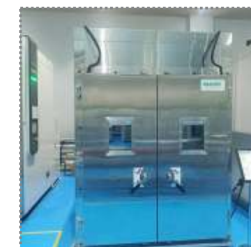
Salt Mist Corrosion Test
