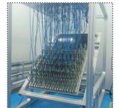
Uniform Snow Load Test
