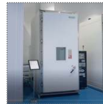
Humidity Freeze & Thermal Cycling Test
