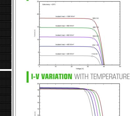
nt Irrad. = 1000 vmm - Cells temp. = 10 °C, Pmpp = 610.5 W - Cells temp. = 25 °C, Pmpp = 585.0 W - Cells temp. = 40 °C, Pmpp = 558.9 W - Cells temp. = 55 °C, Pmpp = 531.9 W - Cells temp. = 70 °C, Pmpp = 504.2 W
